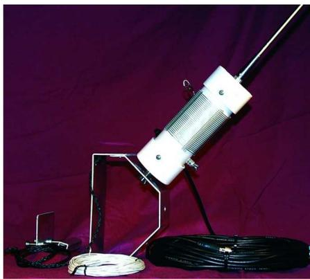
*MFJ-1622 Apartment Antenna covers 40 through 2 meters has smaller telescoping whip, no tuner and retails for \$99.95. (Courtesy: MFJ Enterprises)*
