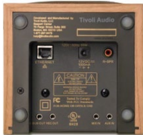
Connections are found on the bottom of this unit instead of on the back for a neater look.
