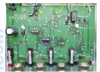
the "none" position, which was indicated as default in the manual, but with our "factory fresh" test sample, for some reason it was set at "moderate." If you are using the whip antenna with the 1026, both stages are used and the jumper is set open (pins 1 and 2 on JMP2).
