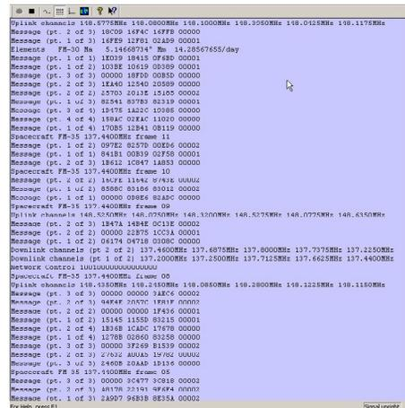
Figure 3 - The message screen. Notice the program-generated downlink frequencies at the bottom; decoded four groups of alphanumeric characters at the top.
