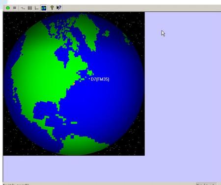
Figure 2 - The chart (map) view showing satellite FM-35's orbital position
