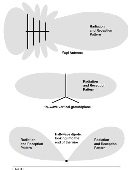
*Antennas are designed to favor certain directions, both for transmitting and receiving. The lower the frequency, the more the signal is capable of following the contour of the terrain, and the less likely it is to be absorbed by trees and foliage. One study showed that with dense trees and vertical polarization, attenuation at 30 MHz is about 3 dB, increasing to 10 dB at 100 MHz.*
