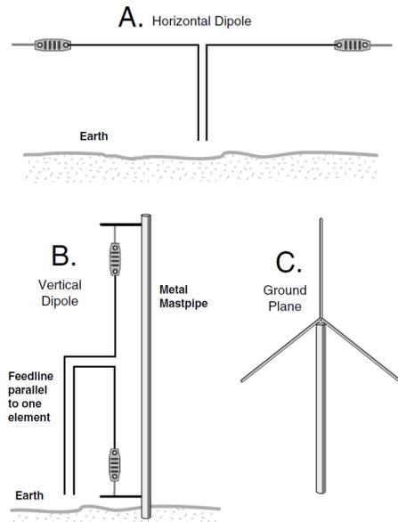
Most vertical antennas are unbalanced, often making use of radial systems as an artificial ground reference. There is nothing inherently superior about one over the other; it is merely a question of whether they are best fed by twin lead (balanced) or coax (unbalanced). Balun (balanced-to-unbalanced) transformers, which we will discuss later, as well as transmatches can be used to match balanced to unbalanced circuit elements, and to match impedances.
