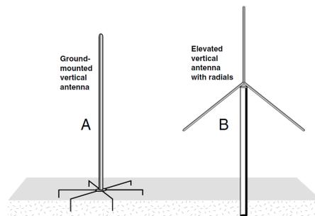
**The radial counterpoise on a ground mounted vertical (A) prevents soil absorption of the radio waves; the radials of an elevated vertical (B) are part of the antenna itself and help shape the pattern.**
