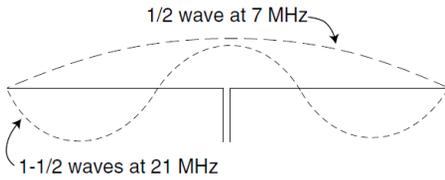
A 67-foot dipole is half-wavelength at 7 MHz, but 1-1/2 wavelengths at 21 MHz. As the frequency increases, wavelength decreases.
