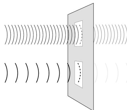
*The higher the frequency, the shorter the wavelength and the easier it is for a signal to get through an opening in an absorptive or reflective enclosure.*
