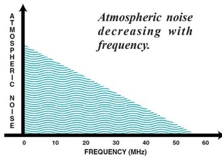
the receiver's own self-generated circuit noise, a larger aperture will only increase the atmospheric noise right along with the signal. If the noise is locally generated (power lines or an electrically-noisy neighbor, for example) a beam or loop antenna can be rotated away from the source of the noise to null the interference, hopefully toward the direction of the signal as well.
