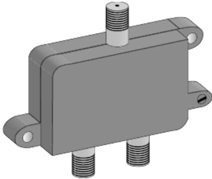
*Splitters are used to feed one antenna to two (or more) receivers; they can also be used in reverse to combine two (or more) antennas to operate one receiver.*
