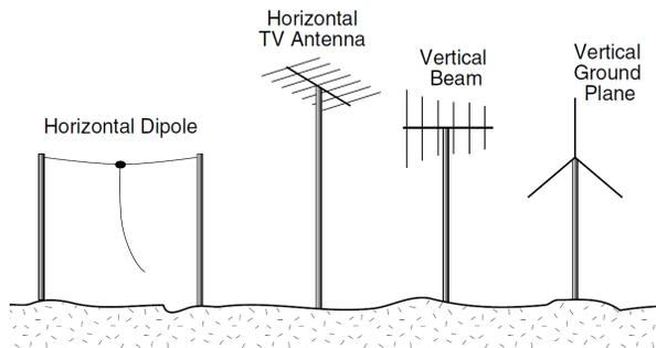
*The polarization of an antenna is simply its relationship to the surface of the earth.*
