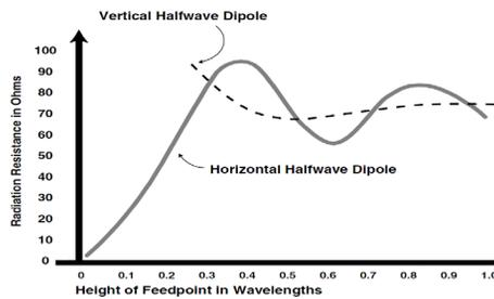
the feed point resistance of a horizontal dipole, typically dropping from 100 to nearly 0 ohms as the antenna is lowered from 0.33 wavelengths to the earth's surface, and fluctuating between 60 and 100 ohms at heights between 0.33 and 1 wavelength.
