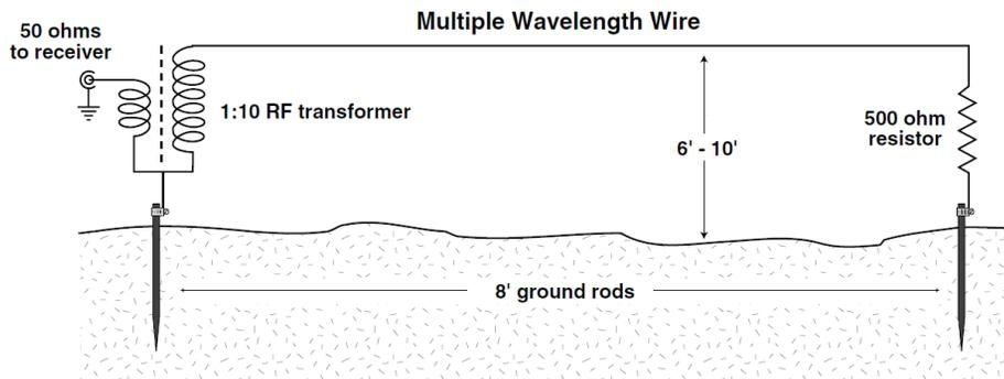
*The Beverage is an example of a high performance, low frequency, grounded receiving antenna.*
