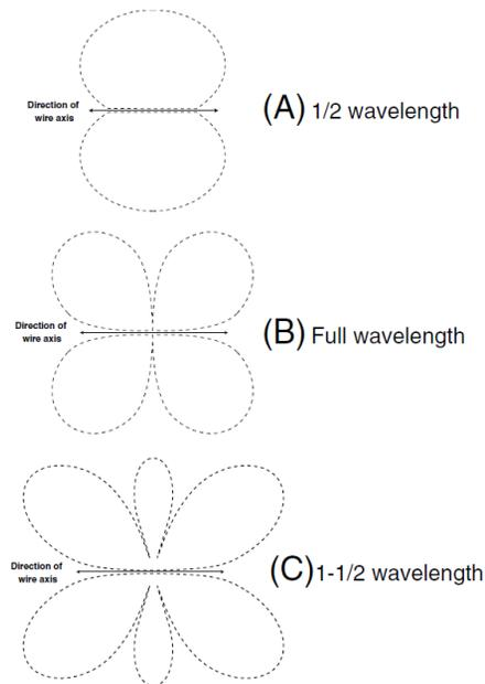
A halfwave dipole (A) as seen from above has a classical figure-eight pattern at right angles to the wire. The same antenna at twice the frequency, now a full wavelength, has a cloverleaf pattern.
