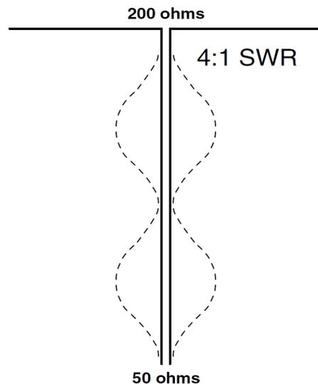
In an unmatched system, line losses are even worse. High-SWR voltages dissipate more power in the transmission line's dielectric (insulation breakdown), current peaks dissipate more power in the conductor (resistive losses) and both effects are aggravated by rising frequency. The result is that power is being wasted as heat.
