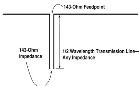
But remember, most antennas exhibit a very narrow frequency bandwidth for a given impedance, so all this magic occurs only around one frequency; on single-element antennas like dipoles and verticals, it also works on odd-harmonic multiples, although the match degrades as we increase the number of multiples.
