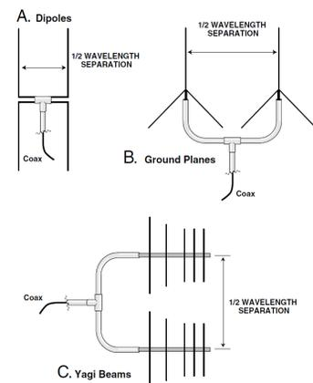
**Stacking any two identical antennas, regardless of their individual gain, will increase the total gain by 3dB.**
