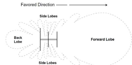
**The Yagi is a popular beam antenna with forward gain.**
