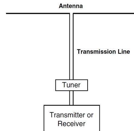
This "tuned feed-line" approach can be used with single wire, open parallel line, twin lead, or coax equally well. Since a transmatch is typically connected between the transmitter (or receiver) and feed line, it can only impedance-match those two points; it has no effect whatsoever on matching the feed line to the antenna. We would need to connect the transmatch between the feed line and antenna feed point to produce a match there.
