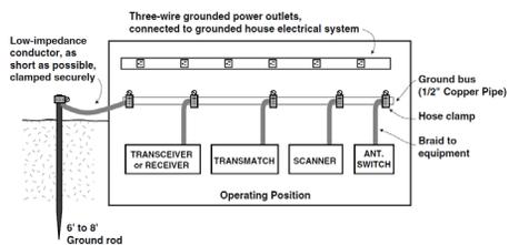
**A good ground system utilizes short, large-gauge wire to connect radio equipment commonly to at least one deep ground rod.**
