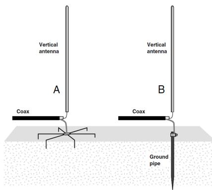
**A good radial counterpoise (A) is always preferable to using lossy Earth (B) in a vertical antenna system.**
