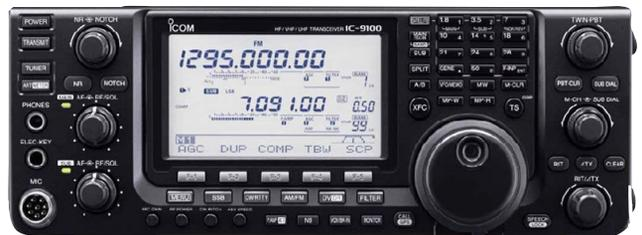
In satellite mode, the ‘9100 will synchronize uplink and downlink frequencies via 20 satellite memory channels that let you store operating modes and tone settings as well as other satellite-unique parameters. As of this writing, sale of the IC-9100 in the United States is still awaiting FCC approval. Retail price, when it finally hits dealer shelves, is expected to be around \$4000.
