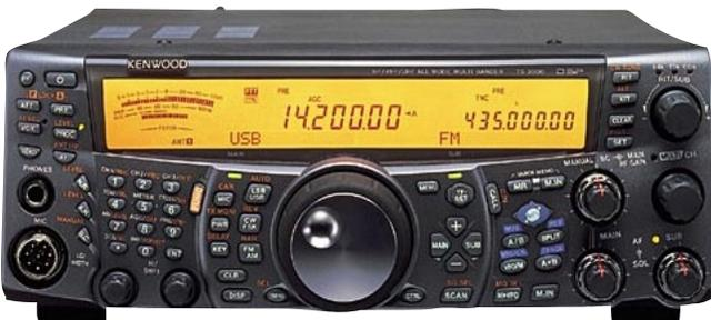
thing” rig, this HF/VHF/UHF all-mode radio has a 100W transmitter for HF through 2m, 50W on 70cm, dual channel receive, digital signal processing (DSP), superb frequency stability, as well as a built-in auto antenna tuner for 160 through 6 meters.
