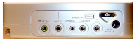
Lots of audio interconnect possibilities, an external AM antenna jack, and an RF gain control.
