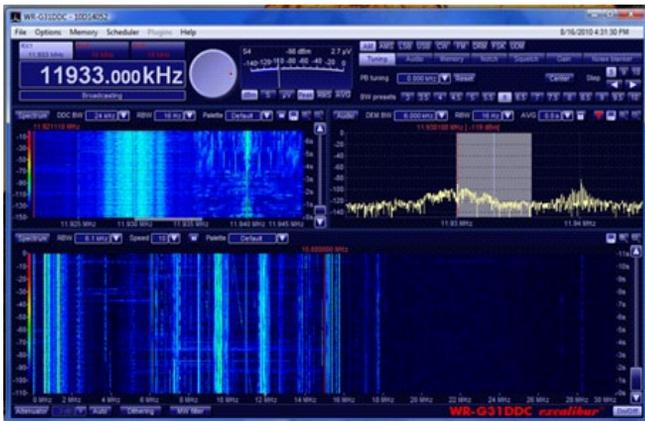
**G31 waterfall displays showing full spectrum users (lower) and modulation patterns on a smaller, magnified portion of the spectrum (upper).**
